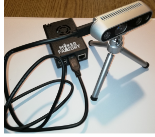
Fig. 3: RPi 4B + Intel D435 camera (RGB-D sensor - fixed node)
