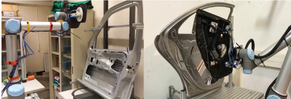
Figure 7: The robot is able to insert the plastic module into the door, both in Stuttgart and the laboratory facility.
