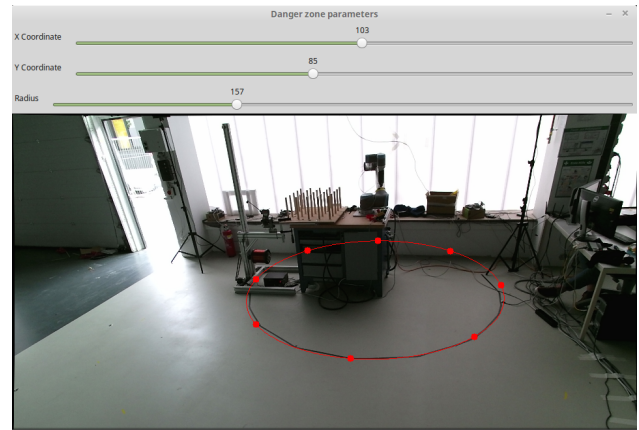
Figure 4. Danger zone calibration. A window let the user tuning the danger zone parameters until is aligned with the tape on the floor.
